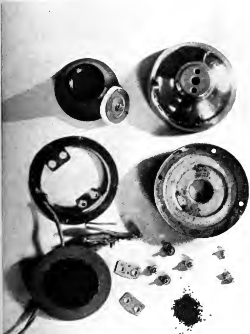
FIG. 42.—WILLIAMS TRANSMITTER DISSECTED.
